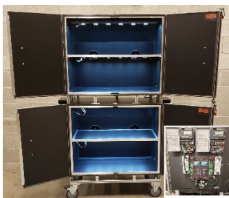
Custom built circadian chambers complete with lighting and timers
